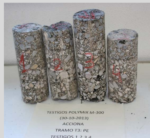
Asphalt mixes (core samples from Pilot)
